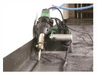
The minimum distance from the wall of only 51 mm allows easy welding of the most common and even vertical junctions gorges. The low height of the unit allows continuous welding since the passage is at least 295 mm height.
