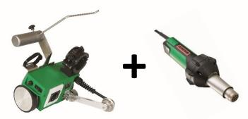
Minifloor turns your hot air blower manual appliance automatic welder Minifloor hot air within a few seconds, which increases the quality of welding, to facilitate the work and significantly reduce the time needed to work. Its use is advantageous from a weld length of 1.20 m and due to its low weight of 5.3 kg it can be transported effortlessly.
